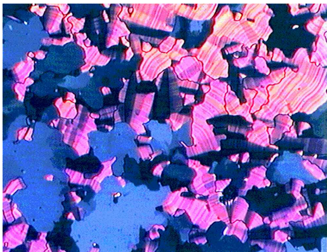
Figure 3. Polarized optical microscopic texture of the induced E phase of the mixture 3b/3a ( x_{3b}=0.7 ) at 158^\circ\text{C} .
